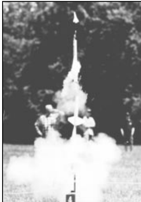
Jonathan Charbonneau's Launch Pad kit spills it's guts after a motor in the cluster fails. (N. Heyen photo)
