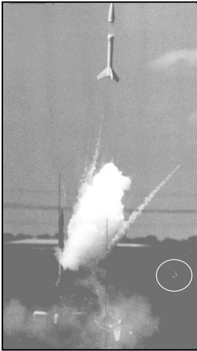
Norm Heyen's Warp-II has a core breach on the pad, but the upper stage ignited and made a safe flight. The booster can be seen at the bottom, and the booster motor mount is in the circle. (photo by N. Heyen)
