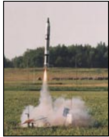
Bob Wiersbe's Gemini-Titan limps off the pad when only one of two motors ignites. (N. Heyen photo)
