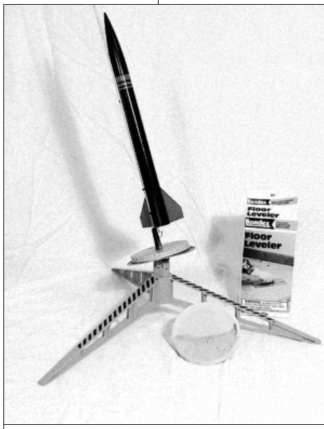
Figure 1. A Standard Launch Pad Equipped With an Ablative Blast Plate
