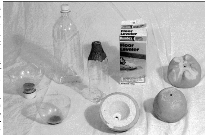
Figure 2. Parabolic and Fluted Ablative Blast Deflectors Left side of picture shows the blast deflector molds. Right side of picture shows finished parabolic and fluted blast deflectors. The underside of cast deflector shown in the middle of this picture.
