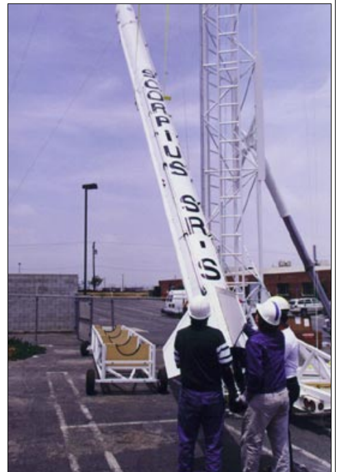
Raising the SR-S to attach it to the launch rail during roll out tests. (Microcosm photo)
