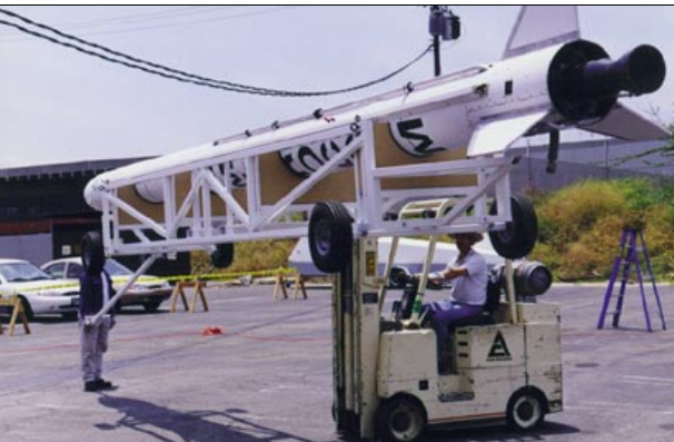
The SR-S and its transport cradle being moved by a standard fork lift during roll out tests. (Microcosm photo)
