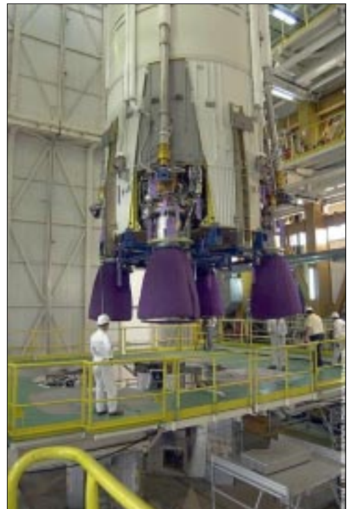
Close-up of Ariane 44L/V148 first stage engines
