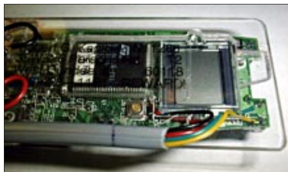
Photo 4: The LCD end of the camera (Rick Gaff photo)
