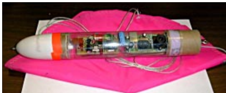
Photo 2: The complete camera in its payload bay (Rick Gaff photo)
