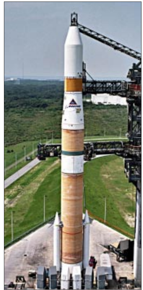
First flight Delta IV unveiled during July RF testing at LC 37B. (Boeing photo)
