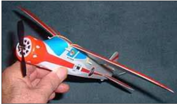
Fig. 1: The Pee Wee Flyer is an RTF electric, all-foam, RC rudder-only plane that uses a 3-cell NiMH pack.
