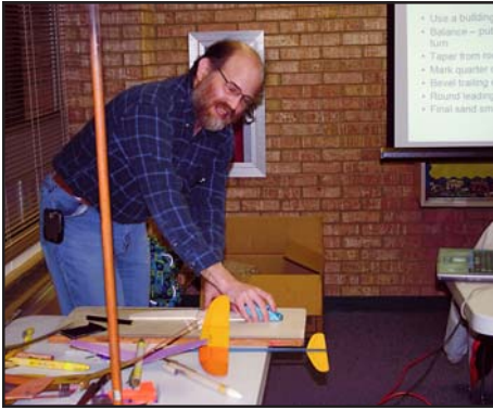
Bob Kaplow shows how to use a razor plane and sanding blocks to properly form an airfoil.
